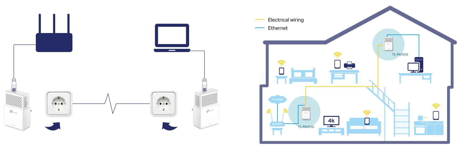
Powerline adapters and extenders must be deployed in a set of two or more.
